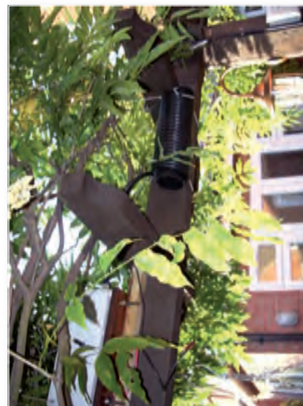
Fig. 5: The choke balun runs down, and is attached to a leg of the pergola.
